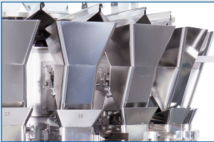
MultiWeigh® "Direct-Drive System", steppermotor operated hoppergates
